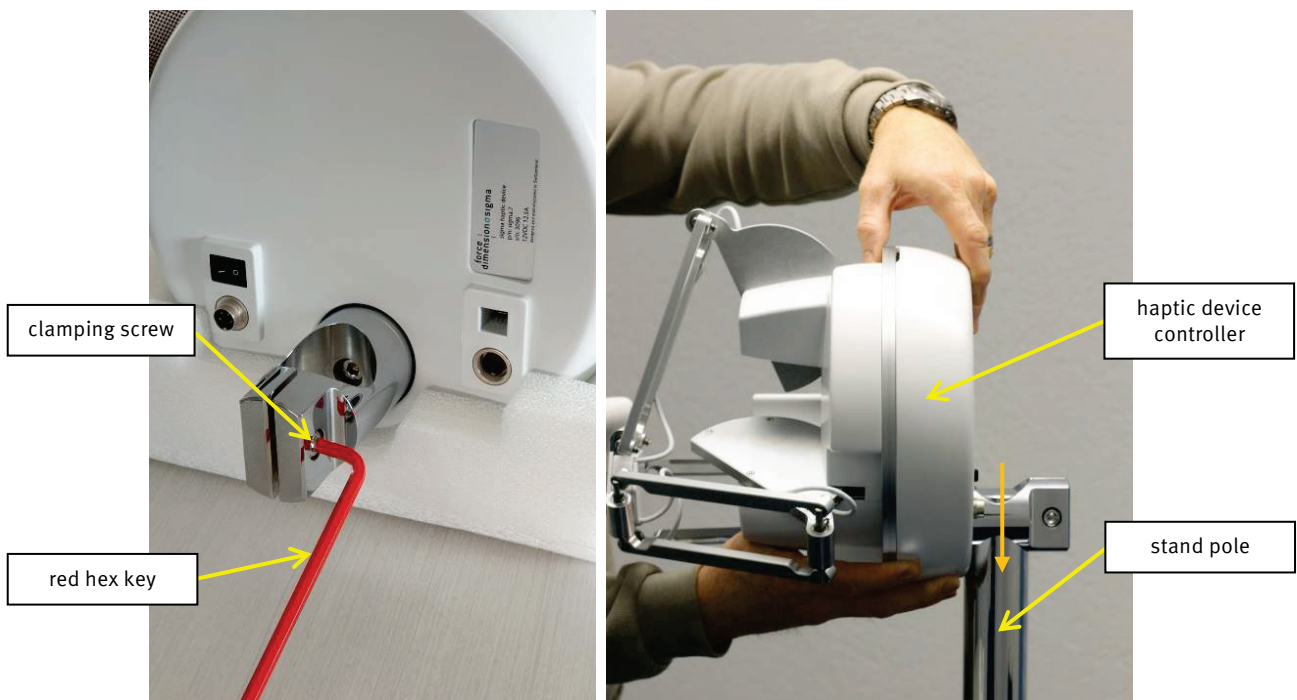
figure 11 – after loosening the clamping screw, the haptic device controller is mounted on the stand pole
